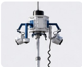
A closer look: dual 4K PTZ cameras, floodlight, and antenna array — 25 ft up.
